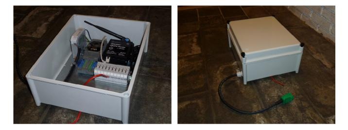
The box containing module for measuring temperatures, power supply and GSM-router.
